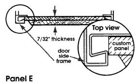
to clear console. Use both hands to bow top and bottom edges of color door panel(s). Remove color panel(s) and spacer. Save color panel(s) and spacer for future use.
